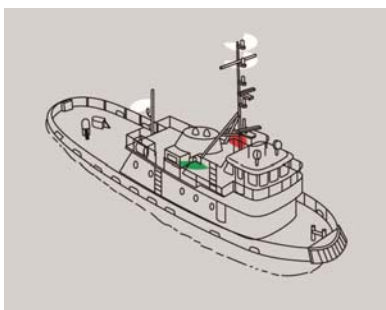
Power-driven vessel pushing ahead or towing alongside— towing vessel less than 50 meters in length. International only.
